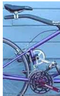
Driving the kid crank from another crank, typical installation & SoftRide setup.
