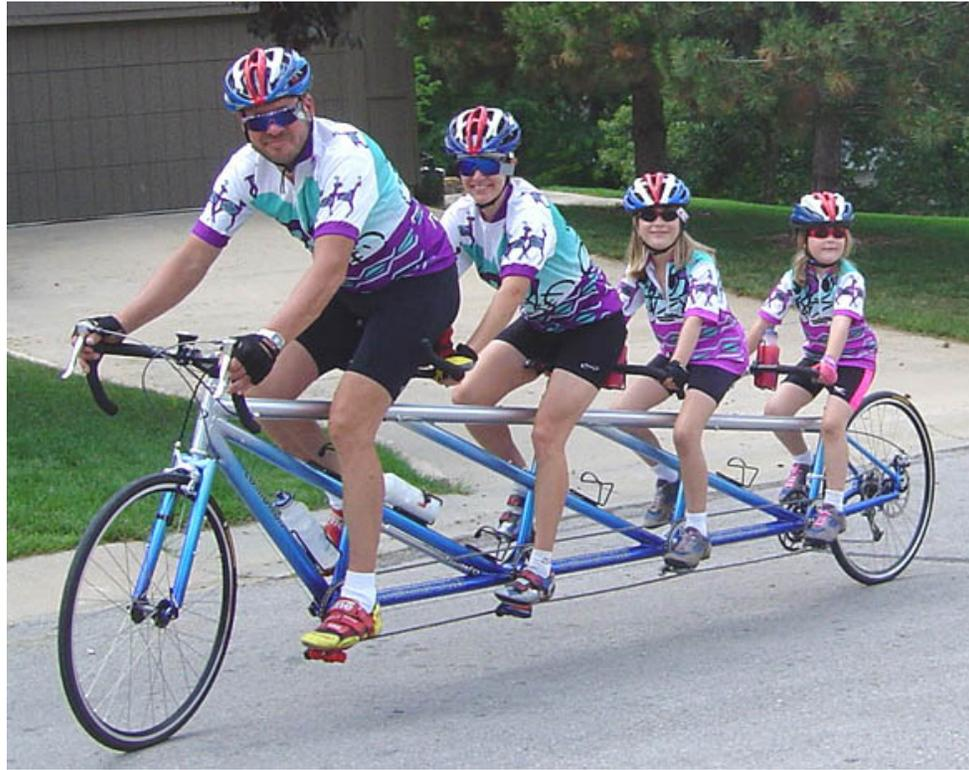
With the right size frame and shorter 125mm/145mm crank arms, child stoker kits are no longer needed even at the age of 5 & 7.5 years. Photo of our Custom Co-Motion Quad taken just before BAK 2005.
